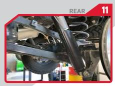
Rotate the shaft so the Falcon logo on the roost guard faces forward.
