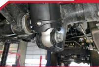
Install the lower end using the factory hardware and torgue to 100 ft. lbs.
