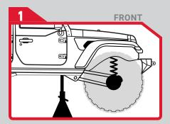
**INSTALL PREP:** Remove the front shocks
