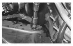
Note: On vehicles equipped with cruise control, you may choose to move the cruise control vacuum diaphragm out of the way by loosening the bolts above the strut assembly on the inside of the engine compartment.
