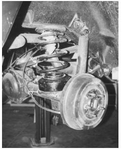
26. Disconnect the rear shocks. If you plan to replace the shock, you can remove the shock completely.
