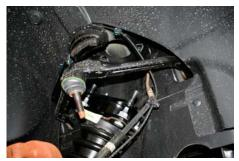
20. Lift the strut assembly into position. Attach the four top
