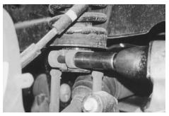
a hammer will cause the A-arm to separate from the knuckle without damaging the boot.
