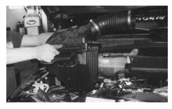
4. Pull the air filter assembly from the vehicle and set aside.
