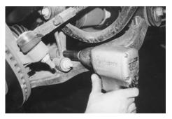
nuts using the new nuts and washers. Reassemble the fork to the bottom of the strut.
