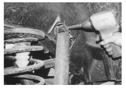
the knuckle. Torque to factory specifications.
