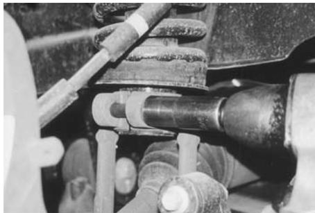
15. Use a 21 mm socket to remove the bolt that secures the top of the fork to the bottom of the strut assembly.
