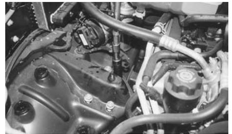
5. Disconnect the upper end of the strut assembly by removing the four nuts that secure it to the body compartment.
