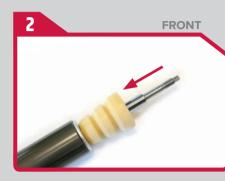
· Orient and install bump stop on shock shaft as shown
