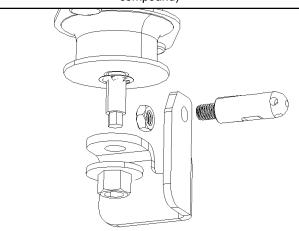
Slide 2.2 assembly onto the body mount and tighten body mount using nut saved from Step 2. Torque to 75 ft-lb (Use thread locking compound)
