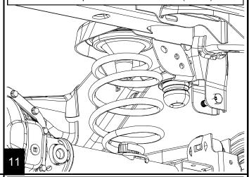
Reinstall the brake lines to the frame. Torque to 84 inch-lbs (9 Nm).
