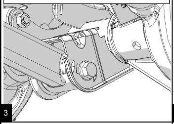
Disconnect the shocks at the axle with an 18mm.
