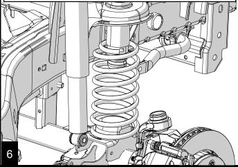
Slide the spacer, then the isolator up the jounce tube, spacer first with the flare facing down.
