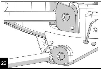
Reinstall the rear track bar at the axle. Have someone push on the body to help align the bolt holes. Torque to 125 ft-lbs. (See 999043 Rear Track Bar/Installation) Recheck every bolt for torque. Re-torque all bolts after 100 miles.
