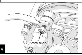
Using the 18mm install the factory hardware and two provided washers on the lower end of the link. Place the washers on either side of the bushing. Torque to 75 ft-lbs.
