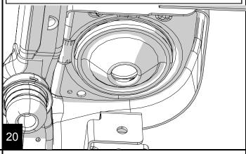
Raise the axle high enough to reinstall the lower shock bolts.
