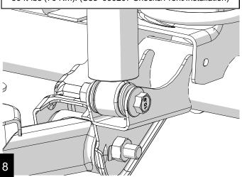
Reinstall the sway bar links or install new links if supplied. Torque top and bottom to 75 ft-lbs. (See 999027 JK Quick Disconnect Links/Installation)
