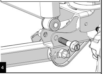
Remove the sway bar links with an 18mm wrench and socket at the axle. If you are replacing the links, remove completely. (See 999027 Front Quick Disconnect/Removal)
