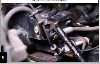
Remove the spring and the spring isolator. Some applications require disconnecting the sway bar links.
