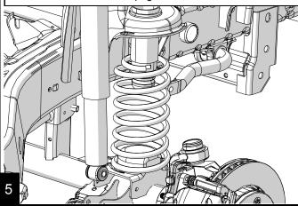
Locate the center of the spring pad and drill a 5/16" hole for standard pad installation. For speedbump pads, drill a 3/8" hole.
