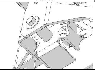
Install the u-bolt around the axle and into the bracket. Torque the nuts to 85 ft-lbs.
