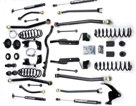
This kit is designed to fit up to 37" tires. Aftermarket wheels with 4.5" backspacing or less is required.
