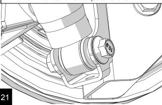
Reinstall wheels and tires, torque to 95-115 ft-lbs. Lower to the ground. Torque all upper control arm bolts to 75 ft-lbs and all lower control arms to 125 ft-lbs.
