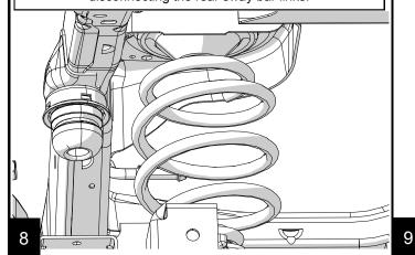
Remove the factory isolator from the upper spring perch and install onto the new spring spacer.
