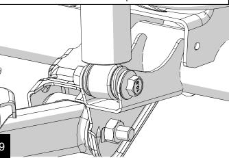
Reconnect the track bar once the vehicle is on the ground. Torque bolt to 125 ft-lbs (170 Nm) Torque wheel lug nuts to 95-115 ft-lbs (129-155 Nm).
