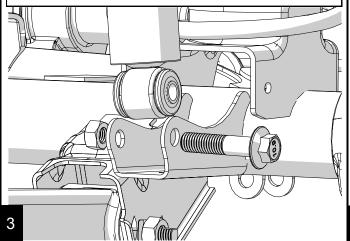
Disconnect the swaybar links front the axle with an 18mm. (See 999027 Quick Disconnect Links/Removal)
