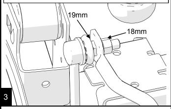
With both factory links removed, install the swivel end of the link into the swaybar from the outside. Install the new lock nut using the 19mm end wrench and the 6mm allen wrench.
