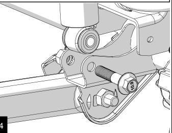
Remove the brake line from the axle side brackets by prying them open. Remove the bracket with a 10mm. Lower the axle until the springs can be removed. Do not overstretch the ABS and breather lines.
