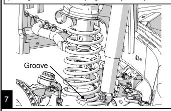
Raise the jack high enough to install the shocks. Torque to 56 ft-lbs (76 Nm). (See 999207 Shocks/Front/Installation)
