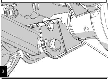
Remove the shocks at the axle with an 18mm wrench and socket. (See 999207 Shocks/Front/Removal)
