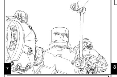
Remove the nut from the front body mount. Insert 2.4 into 2.2. Tighten 2.1.5 onto stud as shown. (Use thread locking compound)
