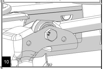
Reinstall wheels and tires. Torque lug nuts to 95-115 ft-lbs. Once the vehicle is on the ground, torque upper control arm bolts to 75 ft-lbs and all lowers to 125 ft-lbs.
