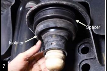
Reinstall the spring. Be sure to seat the bottom of the spring into the groove in the spring pad.
