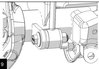
Reinstall the front track bar once the vehicle is sitting on the ground. Torque to 125 ft-lbs. (See 999208 Front Track Bar/Installation)
