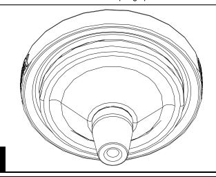
To aid in installation, apply grease to the top of the new spacer. Press the isolator and spacer assembly into the upper spring perch. You can use a piece of wood as a spacer between spring spacer and the axle, then raise the axle to press the spacer in.
