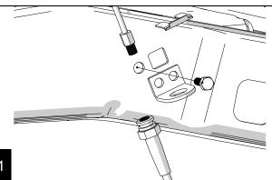
Place a new copper washer on the banjo bolt and insert though the end of the brake line. Place another copper washer between the fitting and the caliper.
