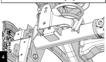
Use the provided sleeve as a spacer and install the 1/2"x3.5" bracket bolt with washers on either side and a locknut. Torque to 75 ft-lbs.
