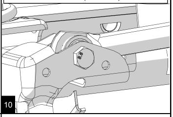
With the jeep on the ground at ride height, torque the upper control arms to 75ft-lbs (102 Nm), the lower control arms to 117 ft-lbs (159 Nm) at the axle and 125 ft-lbs (169 Nm) at the frame.
