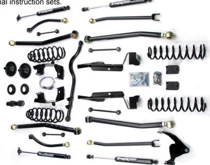
This kit is designed to fit up to 35" tires. Aftermarket wheels with 4.5" backspacing or less is required.
