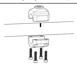
Use a 3/4" to install the remaining end of the stabilizer onto the top of the clamp using the 1/2" bolt and two 1/2" washers. Use Blue Loctite and Torque to 47 ft-lbs.
