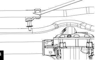
Hint: Slide the stabilizer mount over to the track bar bracket and rotate it until the stud contacts the bottom of the track bar bracket. This will provide a good location to pry on the stabilizer bracket. After prying, slide the bracket to the passenger side of the tie rod. The smaller diameter of the tie rod end will aid in removing the stabilizer mount.
