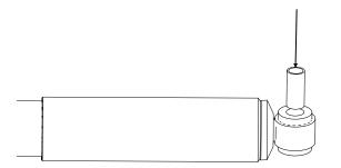
Place the 7/6" Washer on to the new track bar stud.
