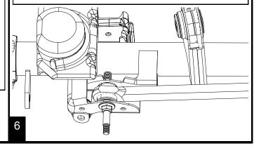
Remove both metal sleeves from the steering stabilizer. Install the supplied 1/2" sleeve (61248) into the piston side of the stabilizer.
