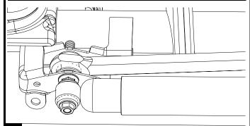
Make sure the tires are straight, then manually collapse the steering stabilizer to its centered position. Hint, use a tape measure. Make a mark on the tie rod where the stabilizer eyelet aligns with the tie rod.
