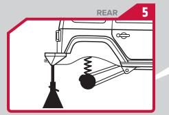
· With rear suspension at full droop remove rear tires (front optional), and existing shocks
