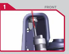
Install tab, bushing, and flat bottom washer first
