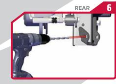
• Drill outside tab only using a 5/8" drill bit Using the softest setting to make the adiustment easie
