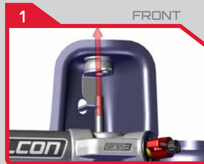
1 FRONT Install tab, bushing, and flat bottom washer first.
