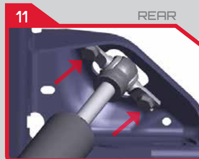
11 REAR Torque both bolts to 30 ft. lbs.
