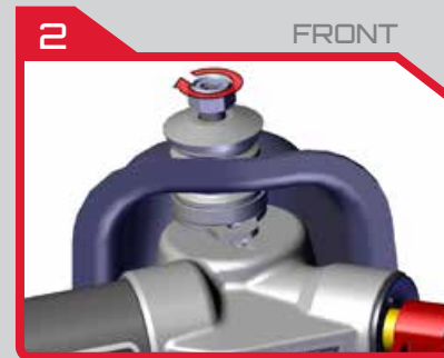
2 FRONT Torque to 15 ft. lbs.
