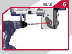
• Drill outside tab only using a 5/8" drill bit Using the softest setting to make the
