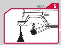
· With rear suspension at full droop remove rear tires (front optional), and existing shocks
