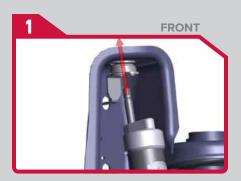
· Install tab, bushing, and flat bottom washer first
