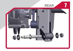
• Torque to 40 ft. lbs. Using 18mm. 6mm hex wrench will prevent bolt rotation
