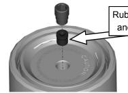
Rubber Plug, lightly oil and small end down
