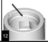
The 8 position and 3 position adjustment pins must both be turned all the way counter clockwise for installation. The outer 3 position adjustment pin can be turned by hand. For the inner 8 position adjustment pin use a 5mm allen wrench.
