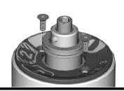
Press cartridge down firmly until it stops, exposing the snap ring groove. Install snap ring into the groove, ensuring the end of the snap ring is just past the notch in housing (see image). This will aid in future disassembly if needed.
