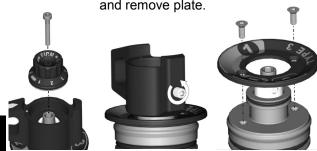
Thread the correct bolt into the center of the cartridge.
