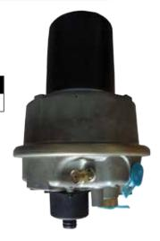
Desiccant Cartridge & Repair Kit Part No. AT6026 Stk. Code 14351
