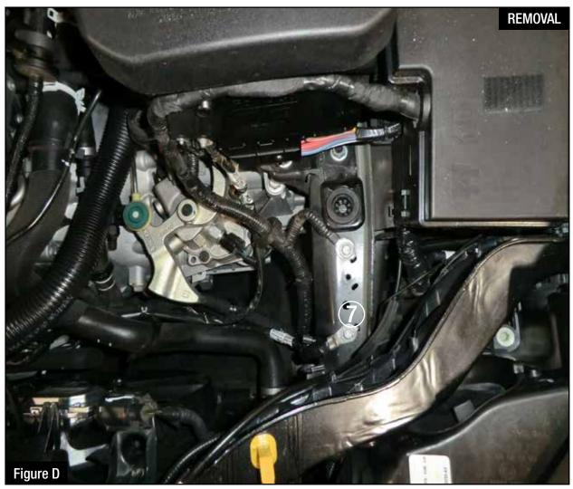
**Refer to Figure D for Step 11** Step 11: Remove the bolt 7 to the ground wires and replace with the M8 isolation mount.
