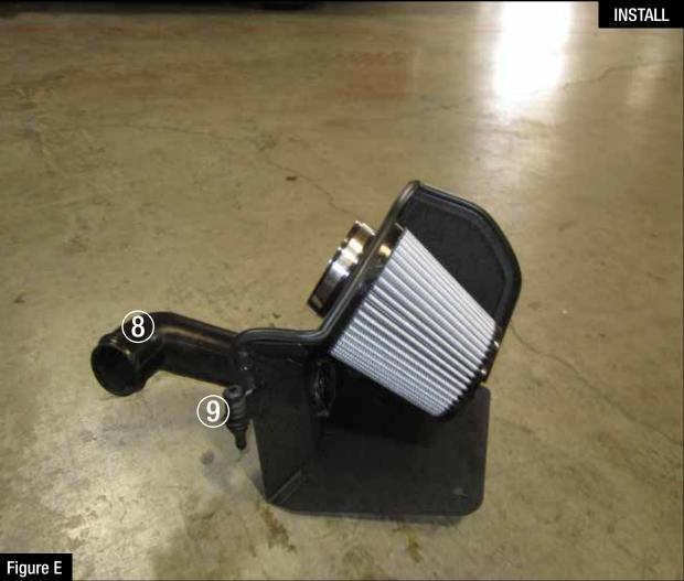
**<u>Refer to Figure E for Steps 12-14</u>** Step 12: Remove the OE air inlet duct (8) off the OE housing and install on the Takeda housing. Step 13: Remove the OE mounting fitting(9) off the OE housing and install on the Takeda housing. Step 14: Install aFe filter onto the aFe airbox housing along with trim seal. Make sure housing is secure in filter retention groove.
