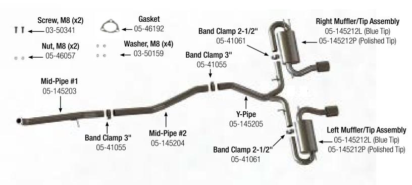
Professional installation is highly recommended. (Read instructions prior to installation). Make sure to always have at least (2) stands or jacks on hand to support the removal of OE system. Also for the installation of aFe system. Any Removal of rubber isolation mounts may require using a spray lubricant such as WD40 and a pry bar.
