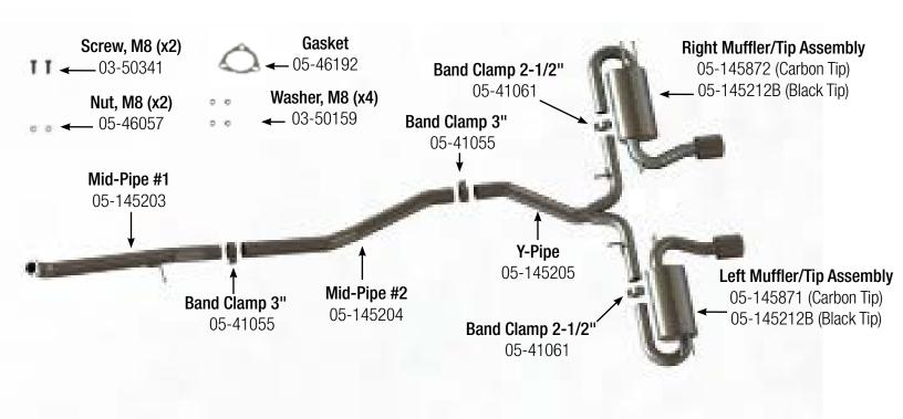
Professional installation is highly recommended. (Read instructions prior to installation). Make sure to always have at least (2) stands or jacks on hand to support the removal of OE system. Also for the installation of aFe system. Any Removal of rubber isolation mounts may require using a spray lubricant such as WD40 and a pry bar.
