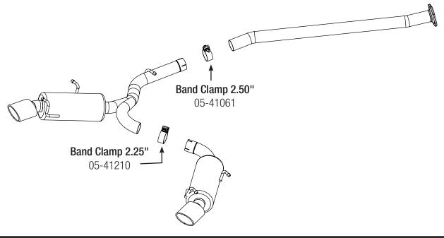
**Caution:** Allow time for your vehicle to cool down prior to installation. When working on or under your vehicle proceed with caution. Exhaust systems reach high temperatures and may cause serious burns. Wear protective safety equipment; eye goggles and gloves to ensure a safe installation.
