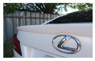
Gently press spoiler into place on the deck lid, hatch or rear glass. Once satisfied with placement, firmly press down on spoiler to ensure adhesion along entire vehicle surface. Continue to apply pressure until satisfied.
