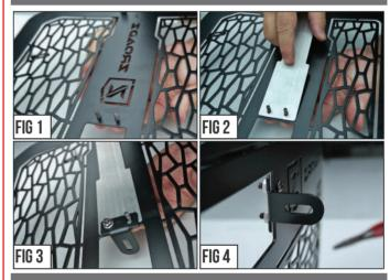
Put into place one of the Bracket Tabs and seucre with STEP 2 provided Hardware as seen in Fig. # 1-4.
