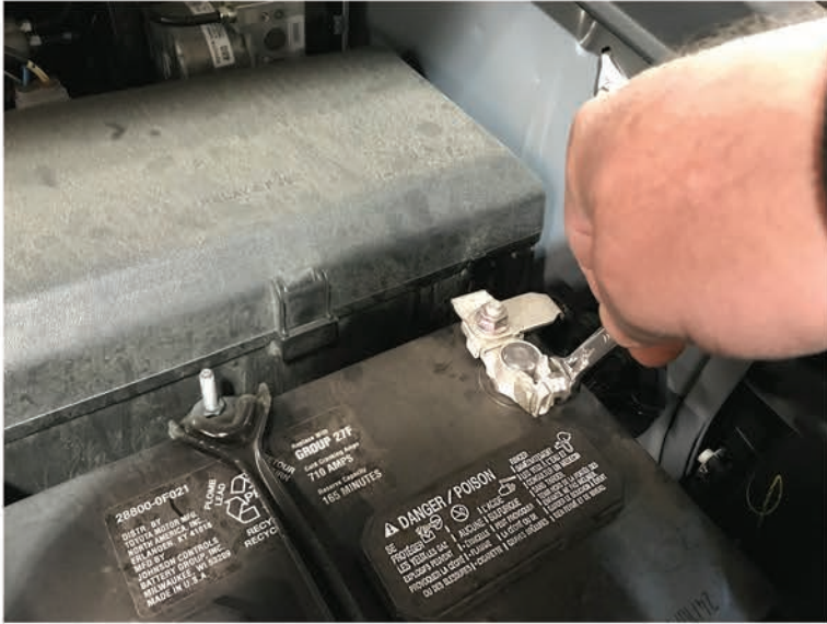
1. Disconnect negative battery terminal.
