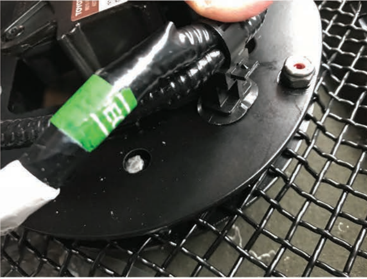
7. Install complete assembly to mounting studs with spacers in place. Use (4) #10 lock nuts and Torque to 30 in- lbs. Note orientation of TOP side of module. Connect harness to module, press harness cable mounts into position as shown.
