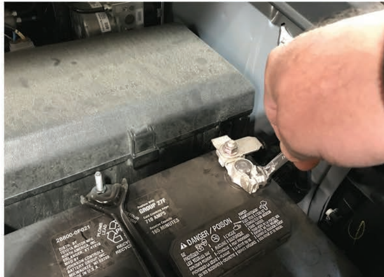
12. Reconnect negative battery terminal.
