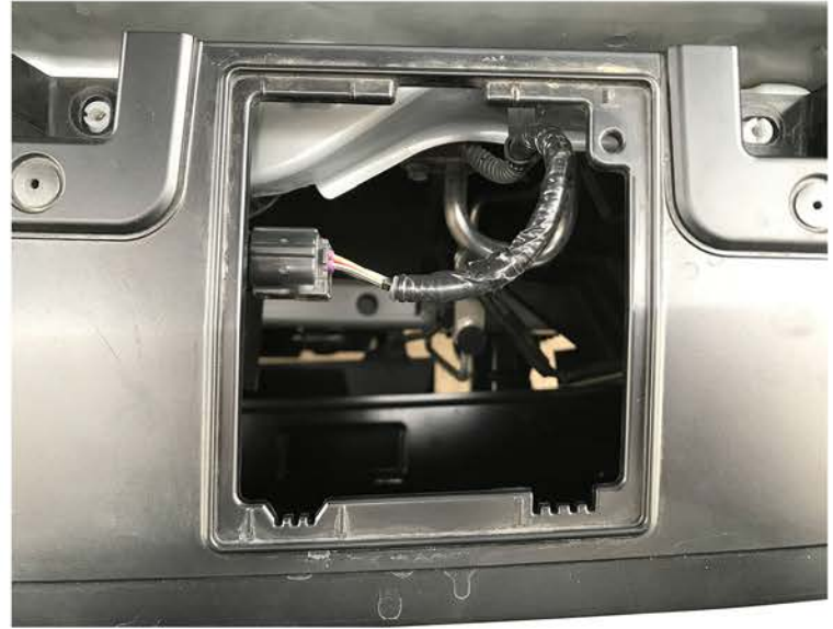
2. Remove access panel (Tundra only) and disconnect TSS harness .
