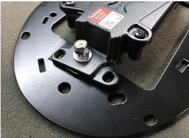
5. Install factory TSS sensor to mounting plate. Use supplied (4) #10 screws, washers and lock nuts. Torque to 30 in-lbs.
