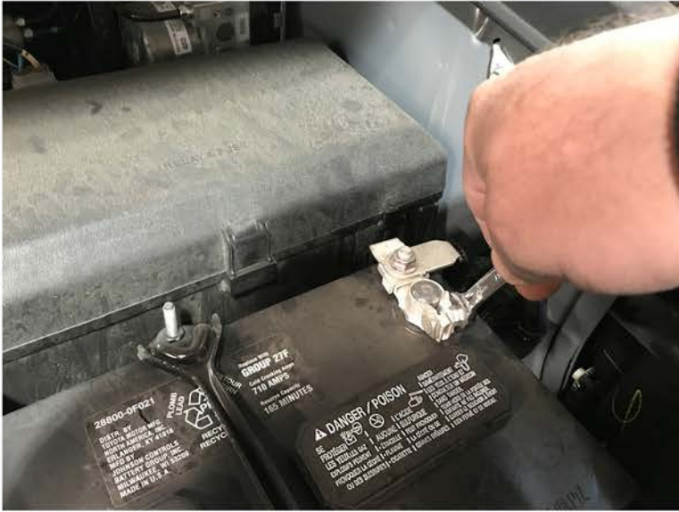
1. Disconnect negative battery terminal.
