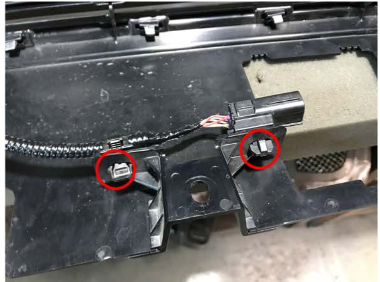
4. Remove harness and connector from factory grille tabs.
