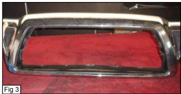
Use a grinding wheel or file to smooth down the areas where you cut out the center section (Fig 4 & 5).
