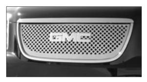
Test fit the insert into the opening; the mounting tabs align to the plastic on top and bottom of the factory grille. Mark these holes to the plastic; drill a  $\frac{1}{4}$ " hole into the plastic.
