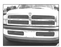
Place each bumper billet in the bumper opening with the brackets on top. The extension brackets attach to factory holes in the bumper. Fasten using the #10 screws and flat nuts. The holes in the brackets are extended so you can adjust the billets in the bumper opening.
