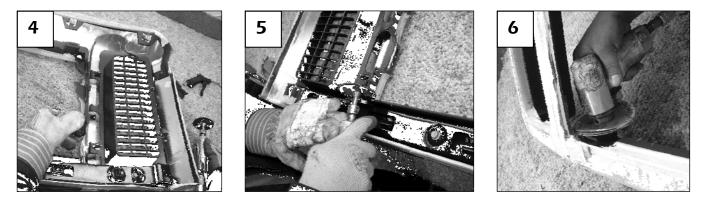
Test fit the center insert behind the OE grille; the ends of the billet bars rest behind the cut edge. Remove any additional material that must be trimmed for installation (4). When completed; the billet will rest flush behind the OE grille opening.
