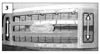
The OE black plastic inserts secured to the side openings (3) must be retained for installation.
