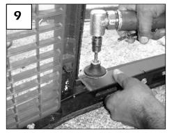
Make additional cuts to finish the required cut edge (8). Use a sanding disc or file to smooth and blend the cuts in each corner (9).
