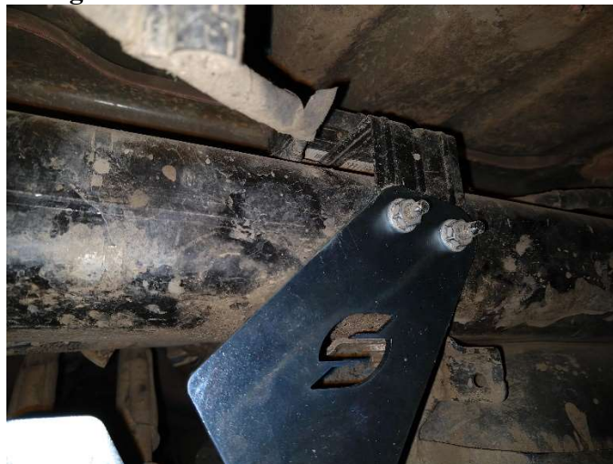
Figure 3. Synergy Parking Brake Cable Bracket Installed
