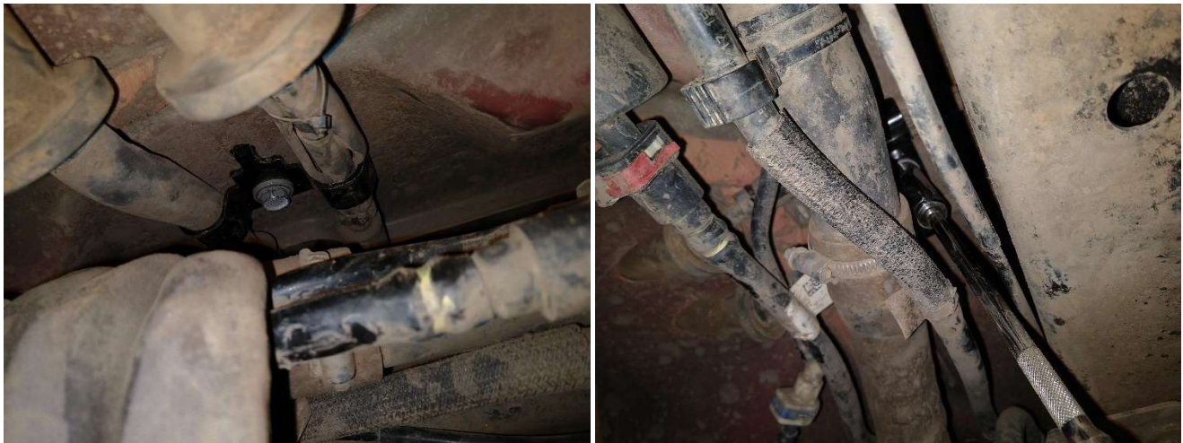
Figures 1 and 2. Removing the Factory Parking Brake Cable Bracket
