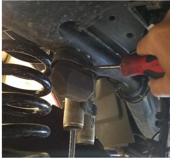
Figure 1. Prying the rubber bump stop out of the mount.
