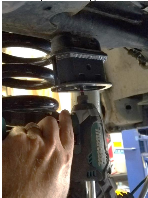
Figure 4. Installing self tapping screw.
