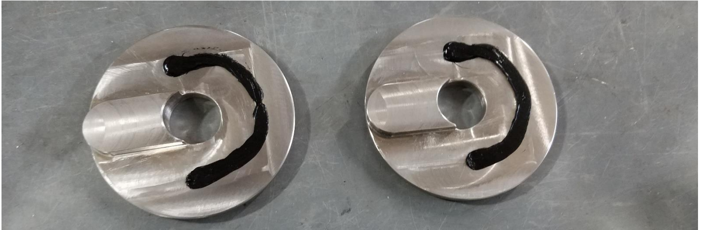
Figure 9. Sealant Applied to Spacers
