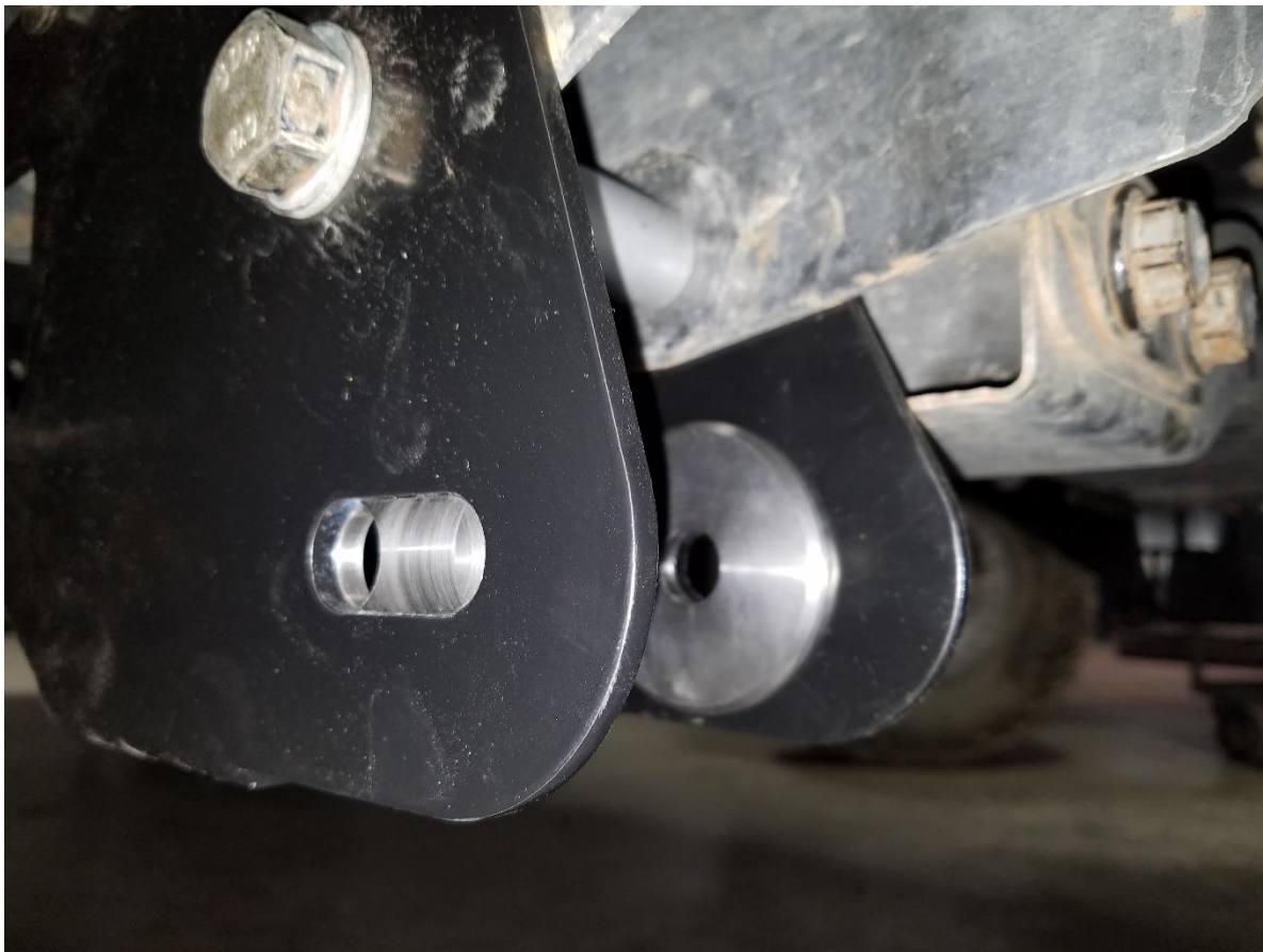
Figure 10. Radius Arm Position Spacers Installed
