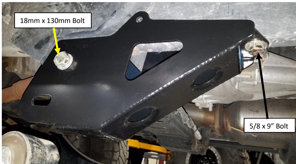
Figure 4. Synergy Radius Arm Drop Bracket Initial Install
