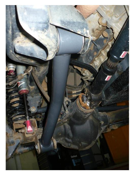
3. Remove the existing lower control arms. If you are just replacing the lower control arms, they can be replaced one at a time with the vehicle sitting on level ground, without removing the tires & wheels or any other suspension part.
