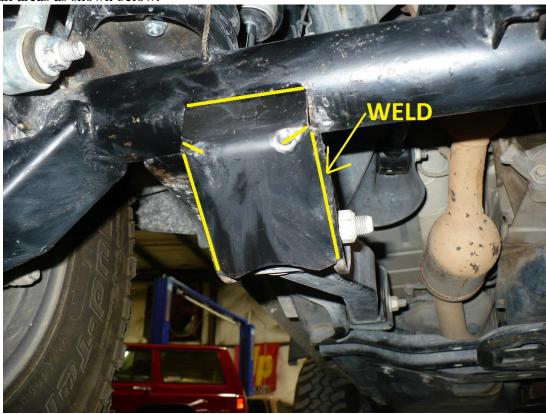
6) After welding, clean off any weld burrs and paint to the desired color to prevent corrosion.
