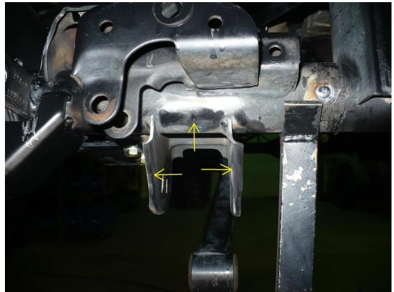
5) Once weld surfaces are prepared, place the LCA skids in position. Tack in several locations and fully weld all areas as shown below.
