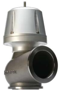
**Synchronic Wastegate WG002** is our large frame universal wastegate with a 50 mm valve and v-band mounting flange that is a bolt-on replacement to the popular 44 mm wastegates on the market today. With each retail kit, you get 4-25 psi of boost in a box.
