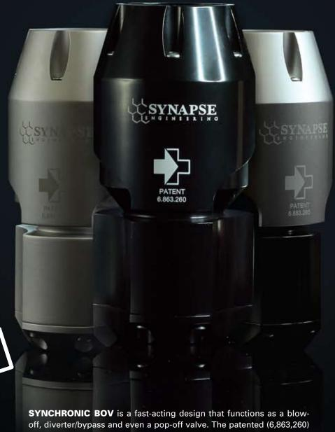
design eliminates the diaphragm with a multi-tier piston actuator that equalizes the force required to open the valve at any boost pressure.
