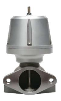
**Synchronic Wastegate WG001** is our smallest frame universal wastegate with a 40 mm valve and 2-bolt mounting flange that is a bolt-on replacement to many wastegates on the market today. With each retail kit, you get 4-25 psi of boost in a box.
