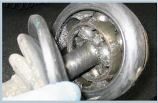
1. Popping or clicking noises when turning. This indicates a worn or damaged outer CV joint. To verify this condition, place the vehicle in reverse, crank the steering wheel to one side and drive the vehicle backward in a circle (check the rearview mirror first!). If the noise gets louder, it confirms the diagnosis and the need for a new replacement CV shaft assembly.
