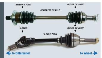
2. A "clunk" when accelerating, decelerating or when putting the transaxle into drive. The noise comes from excessive play in the inner joint on FWD applications, either inner or outer joints in a RWD independent suspension, or from the driveshaft CV joints or U-joint in a RWD or AWD powertrain. To verify the condition, back the vehicle up, alternately accelerating and decelerating while in reverse. If the clunk or shudder is more pronounced, it confirms a bad inner joint.
