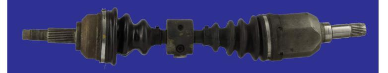
Some OEM axles come from the factory with rubber or metal vibration dampers installed on the center shaft. Dampers are used to combat rotational vibration caused by an axle that isn't perfectly straight or is out of balance at the time of manufacturing. It is proven that after a break-in period, dampers are no longer effective in most cases. An exception to this would be replacement axles for vehicles with adjustable engine mounts such as Chryslers.
