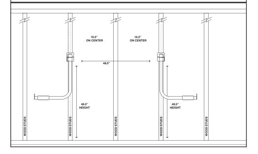
**3** POSITION AND MARK THE APPROPRIATE MOUNTING POSITION. USE THE BRACKET FOR REFERENCE AND DRILL FOUR 1/4" PILOT HOLES IN THE CENTER OF EACH STUD. MAKE SURE PILOT HOLES ARE AT LEAST 2" INTO THE STUD.
