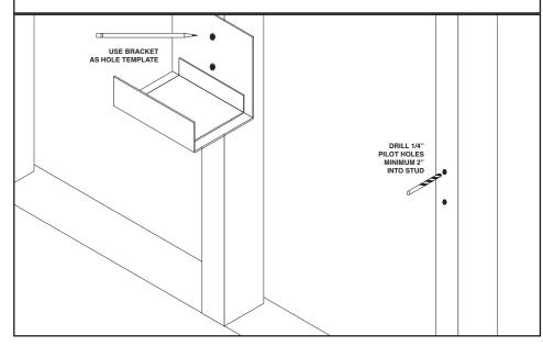
**4** DETERMINE THE PROPER LENGTH 5/16" LAG BOLTS FOR YOUR APPLICA TION. BOLTS MUST BE EMBEDDED AT LEAST 2" INTO STUD. USING 5/16" LAG BOLTS AND 5/16" FLAT WASHERS, ATTACH THE DOOR HOLDER BRACKET TO THE WALL.
