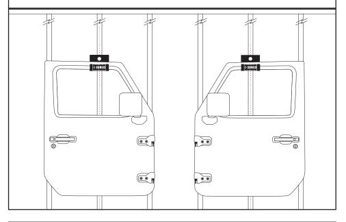
**B** WITH THE WINDOW DOWN ON THE DOOR, THE ENTIRE DOOR VIA THE DOOR WINDOW FRAME CHANNEL (THE RUBBER WEATHERSTRIPPING GAP THAT THE WINDOW GLASS SLIDES INTO) CAN REST ONTO THE END OF THE DOOR HOLDER BRACKET.
