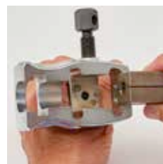
Magnetic yoke holds dies securely in place
