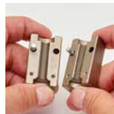
Pins ensure accurate alignment of dies
