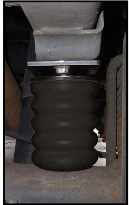
Rear SumoSring SSR-302-47 Installed
