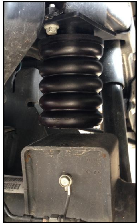
Rear SumoSprings SSR-302-47 installed
