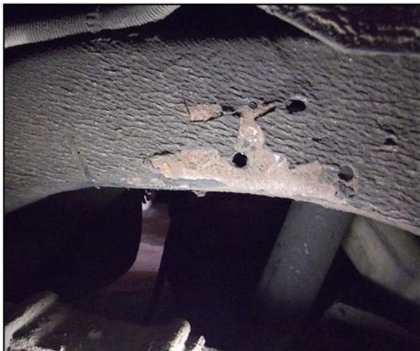
Factory bumpstop bracket removed
