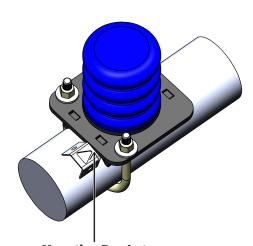
Mounting Bracket should be up against the wire harness bracket. Confirm that wiring is not streched or pinched.
