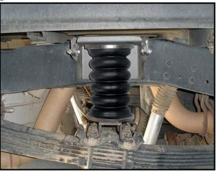
Typical SSR-101 installation with standard lower bracket
