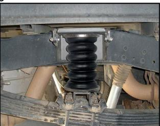
Typical SSR-101 installation with standard lower bracket
