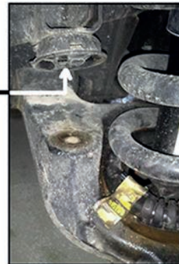
OE Bumpstop removed
