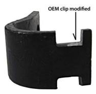
1/8" of clip slot removed for thicker SuperCoil installation
