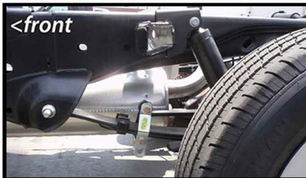
Front shackle install in top hole
