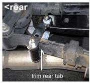
Adjust preload & ride height, select upper shackle hole for heavy applications front ~ spring eye bolt threads out
