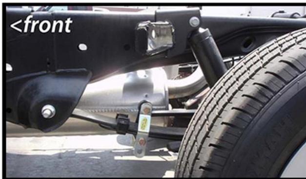
Front shackle install in top hole
