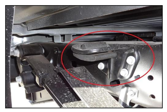
**Step 4:** Place PSP-7 on top of factory spring plate so that it locates on center bolt and spring pad as shown. Place lockdown kit u-bolt on TOP of the PSP-7 between the center and forward bumps. Slip SuperSpring through wheel well or slide in from behind vehicle, positioning it on top of the PSP-7. Position lockdown kit u-bolt with the threads pointing up, install the clamp and thread nuts lightly onto u-bolt. (see pictures below)
