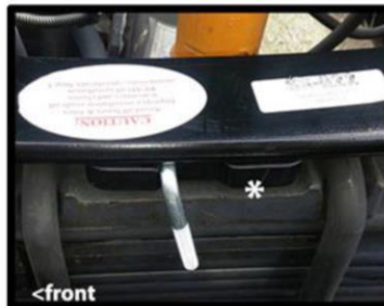
Place PSP11 on top of spring plate flat side up facing, with groove toward the front
