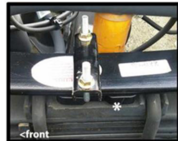
Install the SuperSprings as pictured below, then thread the channel crossplate on to the ubolt. Tighten securely.
