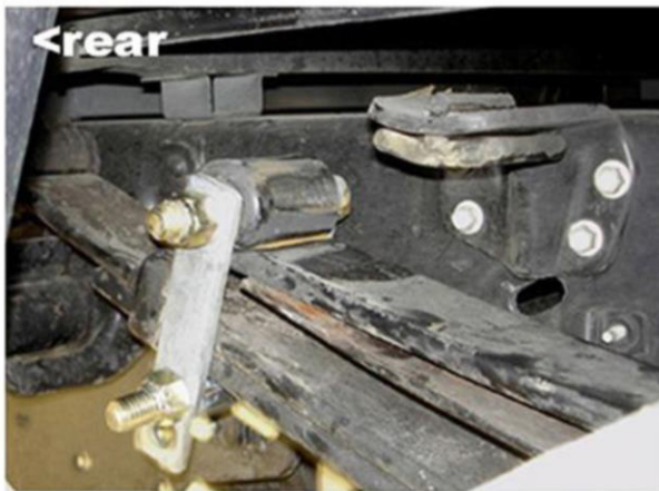
adjustable spring pre-load & ride height
