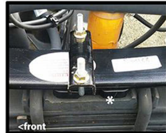
Install the SuperSprings as pictured below, then thread the channel crossplate on to the ubolt. Tighten securely.
