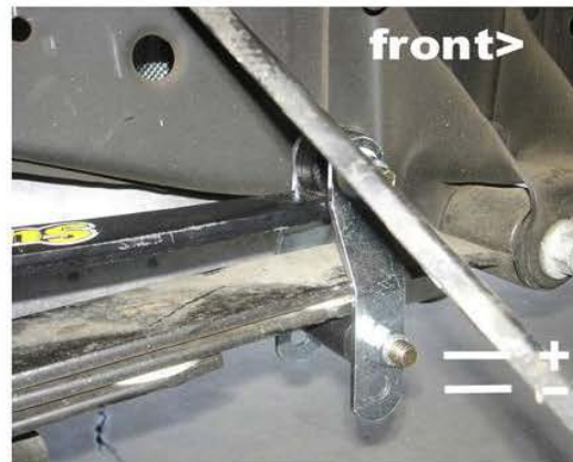
center install hardware clear of factory sensor at axle rear
