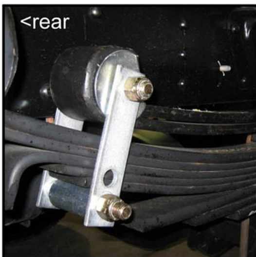
Place PSP11 on top of spring plate flat side up facing, with groove toward the front
