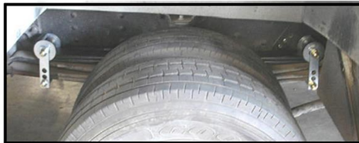
Place PSP11 on top of spring plate flat side up facing, with groove toward the front
