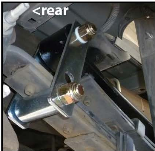
Place PSP 19 on top of spring plate flat side up facing, with groove toward the front
