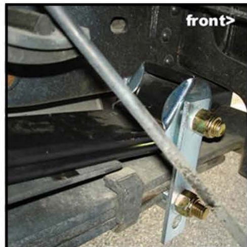
Front & Rear ~ mount spring with eye bolt threads out
