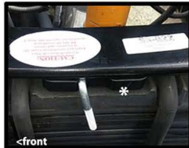
Place PSP 19 on top of spring plate flat side up facing, with groove toward the front
