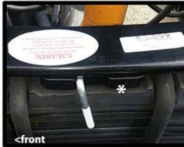
Place PSP-19 on top of spring plate flat side up facing, with groove toward the front
